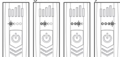
When paired with a Spektrum Smart ESC and compatible receiver, the aircraft battery voltage will be displayed on the DXS transmitter's four LEDs. When in normal operation with a Smart ESC, one LED will illuminate for a low battery, two for a half charged battery, three for a battery between half and full, and four for a fully charged flight battery.
