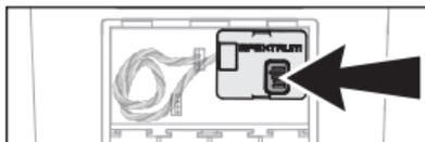
3. Put the student transmitter into Bind mode. The orange LED on the remote receiver will remain lit when it is bound to the student transmitter.
