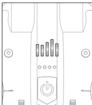
The RGB LED on the transmitter will illuminate green to indicate the transmitter is in trim programming mode.
