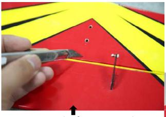
Use a art knife cut open the hole which threading the tail wheel wire and located on horizontal stabilizer.
