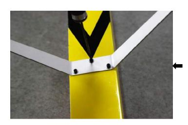
2. Use 2.5mm hexagon socket head screw driver remove the screws
