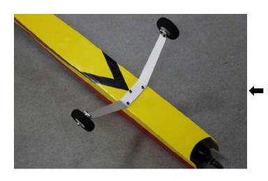
3. Align the landing gear according to the hole position and tighten the three screws
