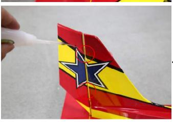
4. Use 502 gluing and fixing it.
