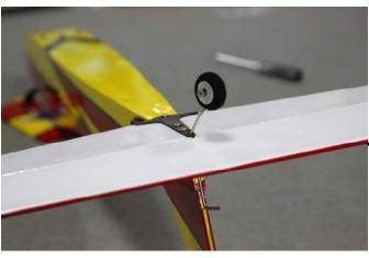
2. Threading the tail wheel wire from the bottom to the top
