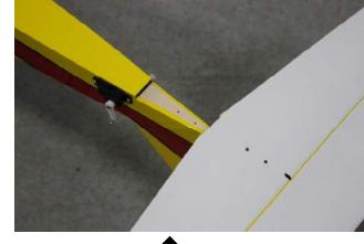
3. Stick the carbon plate to the horizontal stabilizer and screw on three cross-screws
