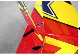
3. Stick the rudder into the tail wheel wire, and insert the rudder hinge into fuselage hinge slot
