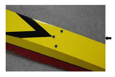
The main landing gear fixing screws have been pre-installed on the fuselage
