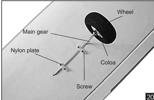
4) Install two of the wheels onto the axles using the four wheel collars and set screws provided. The wheels should be centered on the axles with a wheel collar on each side, holding them in place. Tighten the set screws on the collars to secure them in place. The wheels should rotate freely. You should apply a small drop of lock-Tite thread lock to each set screw to prevent them from coming loose.
