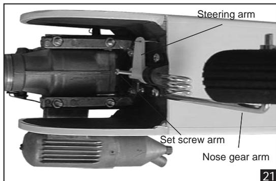
8) With the nose gear wire straight, angle the nylon steering arm about 30° forward of the fire-wall and tighten the set screw. Angling the arm forward like this will allow room for the arm to move back for more adequate steering.
