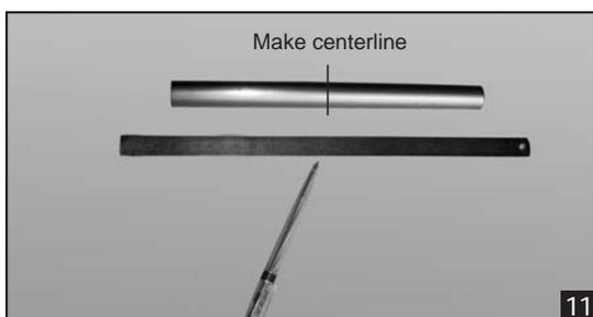
2) Test fit the dihedral brace into each wing half. The brace should slide in easily up to the centerline you drew. If it does not, use 220 grit sandpaper with a sanding block and sand down the edges and ends of the brace until the proper fit is obtained.
