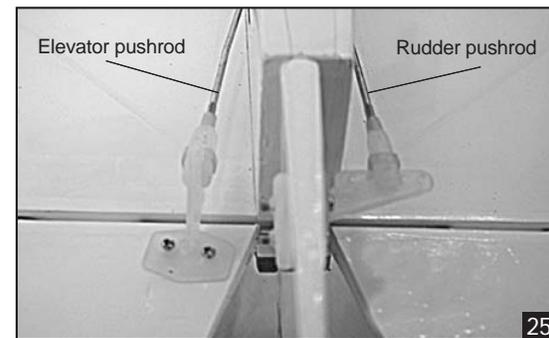
6) Repeat steps 3-5 above for the rudder pushrod. Will exit out the left side of the fuselage. **See photo #19 above.**
