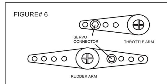
8) Connect the servo to your radio's receiver and turn on the system. Set the trim tabs on the transmitter to neutral and center the servo arms. The elevator and rudder servo arms should be perpendicular to the servos. For the throttle, we suggest setting the throttle trim tab and the throttle stick to the lowest setting which will be used to shut off the engine. Also mount the servo arm about 45° back from perpendicular. **See photo # 7 below.**
