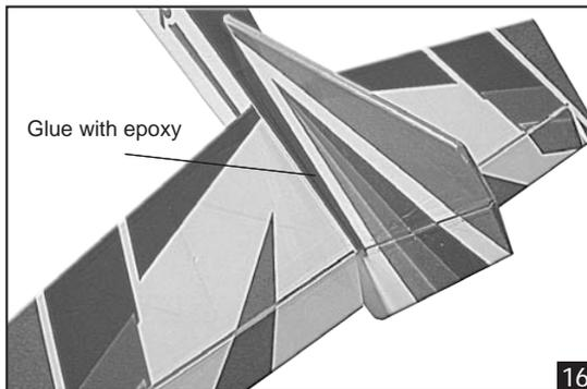
9) Set the vertical stabilizer back in place. Using a triangle, check to ensure that it is 90° to the horizontal stabilizer.
