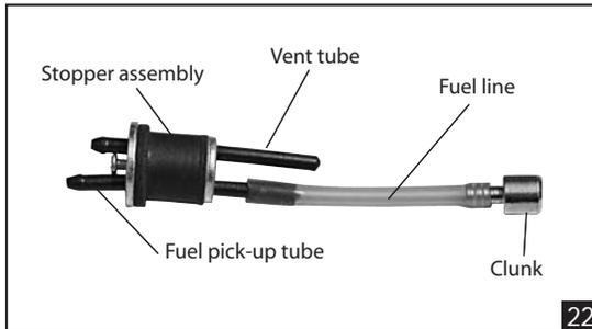
2) Attach the weighted pick-up, more commonly referred to as the "clunk", to one end of the silicon fuel line.
