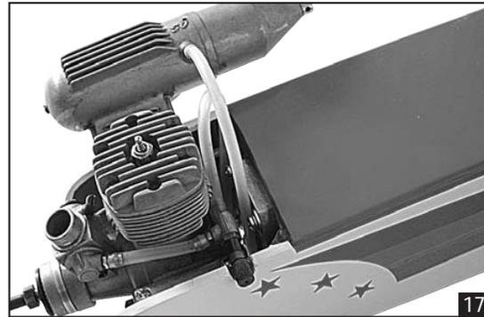
5) Mount the muffler to the engine using the mounting bolts provided with your engine.
