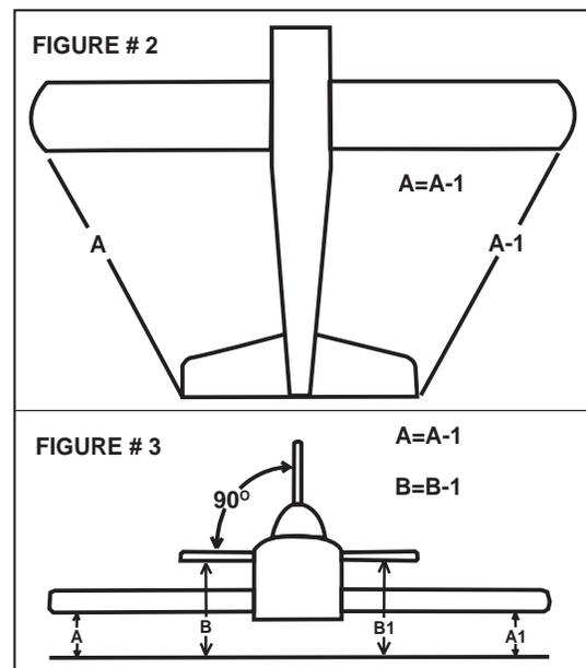
3) When you are satisfied with the alignment, hold the stabilizer in place with T-pins or masking tape, but do not glue at this time.
