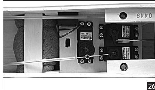
14) Insert the nosegear pushrod wire through the adjustable servo connector on the rudder servo arm. Hold the nose gear assembly in the neutral position and tighten the set screw in the servo connector. Roll the airplane on the ground to ensure it rolls straight. If not, adjust the pushrod wire. When satisfied, cut off the excess wire.
