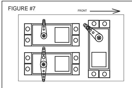
9) One at a time, hold the pushrods in position over the respective servo to check for proper servo direction. If any servo turns in the wrong direction, switch your radio's reversing switches as necessary to achieve the correct direction.
