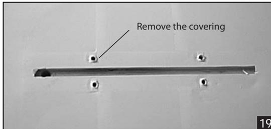
3) Test fit the two main gear wires into the channels. When satisfied with the fit, secure the wires in place using the four nylon straps and eight 3\*12mm sheet metal screws. If you look closely at the wing surface surrounding the channel for the wire, you will notice that there are already four pilot holes drilled to accommodate the screws for the straps. Mount the straps at these locations. **See photo # 14 below.**
